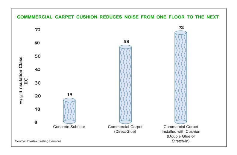
"The absorption co-efficient differences between carpets lies with the type of pile and its thickness. These important carpet features were borne out in the current study, as were cushion density, thickness and porosity."
